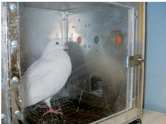
Figure 1 Pigeon in a Skinner box. By pecking on the illuminated disks (response keys), the pigeon occasionally gains access to food delivered in the feeder (opening below the response keys).
